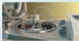
Liquid temperature sensor for more precise liquid temperature control
